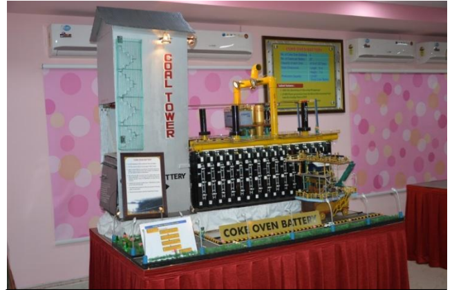
Coke Ovens: The model of the Coke Ovens Battery is useful in explaining the main features of the coke ovens like the no. of batteries, chambers, height, pusher car, charging car, coal tower etc.
