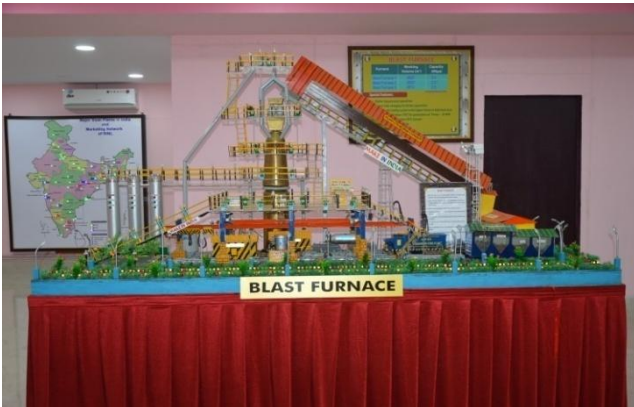
Blast Furnace: The model of the Blast Furnace is useful to understand the features of the Paul Wurth Bell Less Top charging system, Hot Gas blowing through the tuyers, tap holes and tapping system using drilling machine, the use of mud gun for closing the tap hole, runners, rocking runners, ladles, etc.
