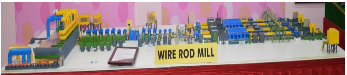
Wire Rod Mill: The model of the Wire Rod Mill explains the process of making various types of wire rods from the point of receiving billets from LMMM and reheating them and then passing them through various sizes of rollers till the final coils are finished and sent to the bundling and packing zone.
