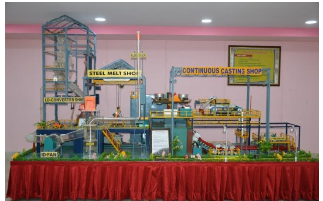
Steel Melting Shop: The model of the Steel Melting Shop will be helpful in understanding the process of steel making like reduction, lancing, scrap charging, Hot Metal charging, Continuous Casting, blooms making etc.
